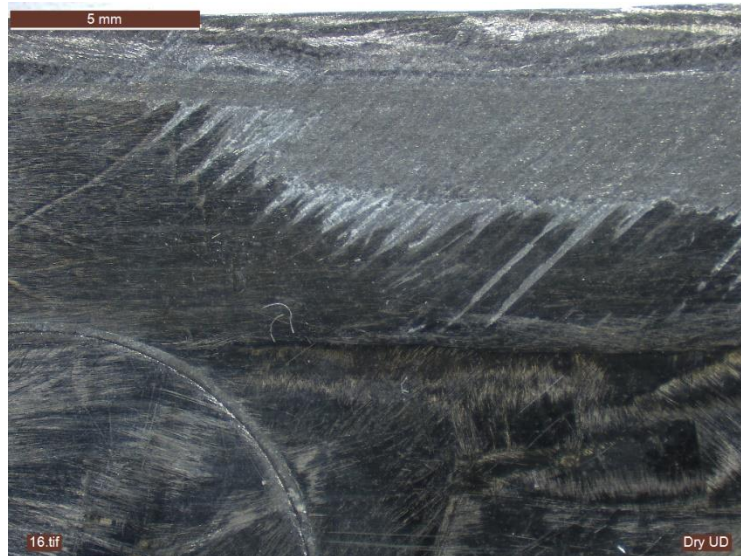
Figure 73: Dry Region from Resin Squeeze Out
