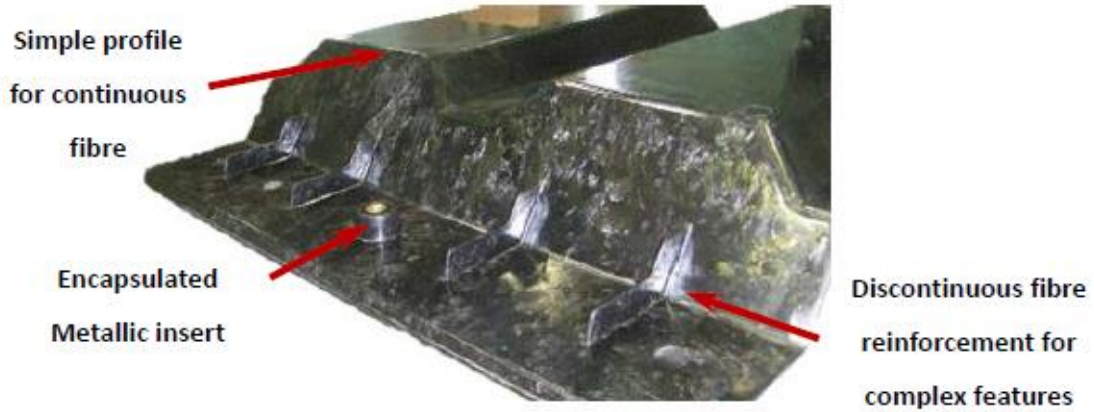
Figure 13: Mitsubishi Rayon Hybrid Structural Floor (Corbridge, 2018)
