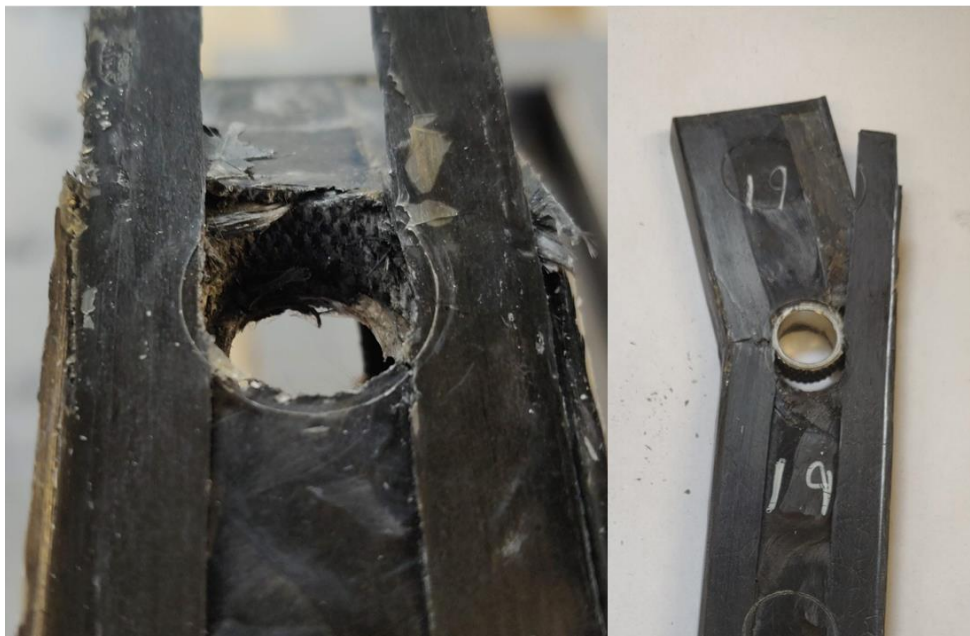
Figure 83: Gripping Effect of the Knurled Insert
