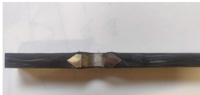
Figure 76: Fibre Flow around Flying Saucer Insert
