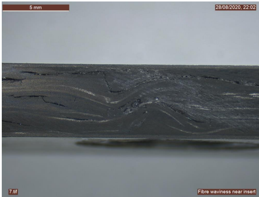
Figure 75: Fibre Waviness near Insert
