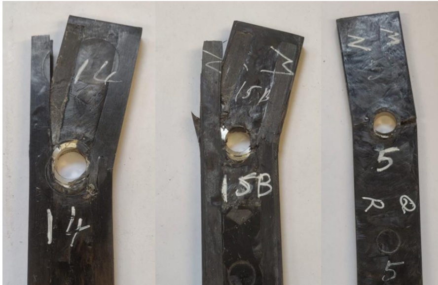
Figure 78: Asymmetric Failure of Specimens
