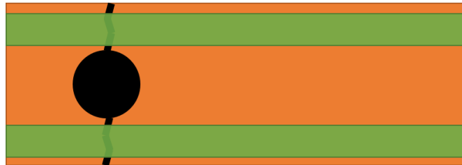
Figure 51: Net Tension Failure of Hybrid Specimen
