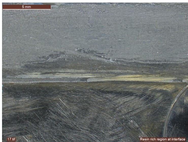
Figure 74: Resin-rich Region at the UD-SMC Interface
