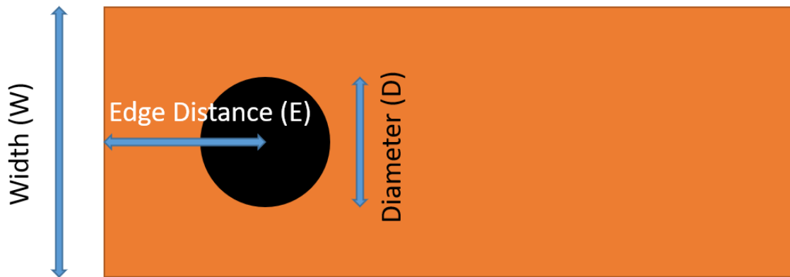
Figure 16: Diameter, Width and Edge Distance of a specimen
