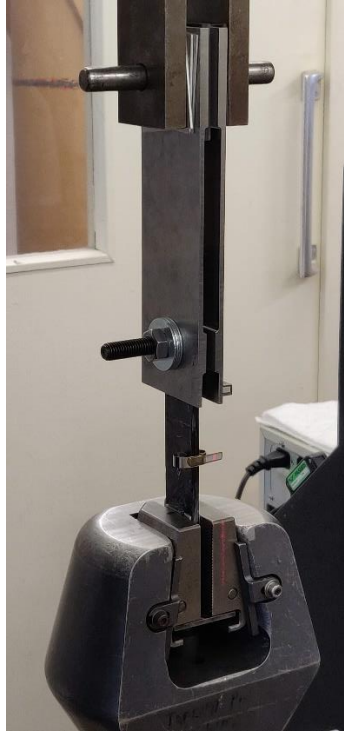
Figure 69: Pin-Bearing Test Set Up
