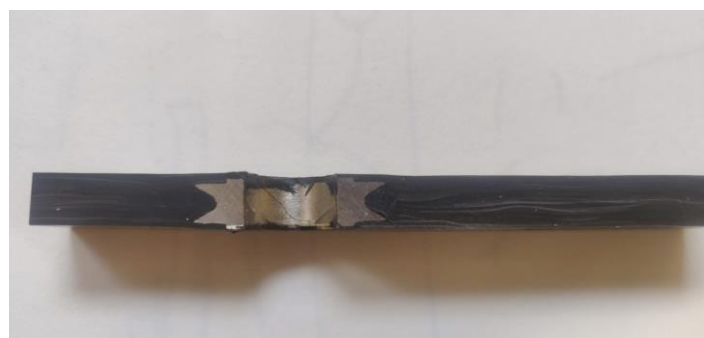
Figure 77: Fibre Flow around Yoyo Insert
